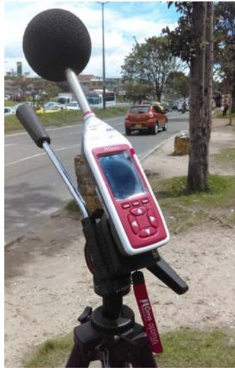
**Figure 2.** Measuring instrument in Ciudad de Cali Avenue (CIRRUS Research plc, 2017)
