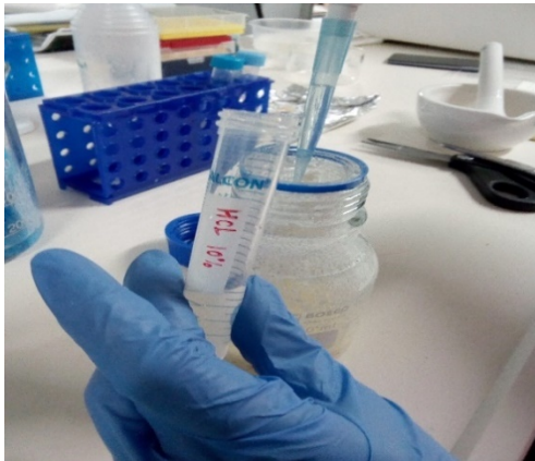
Fig 19 Adding HCL 10% to autoclave method sample Source: The author 2021
