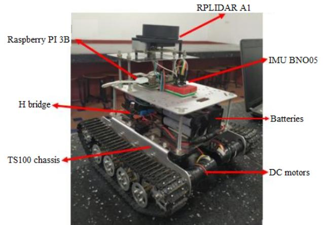
**Figure 1. Mobile robot prototype**
