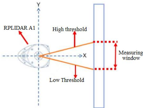
**Figure 2. Window measuring  $e_\psi = 0$**
